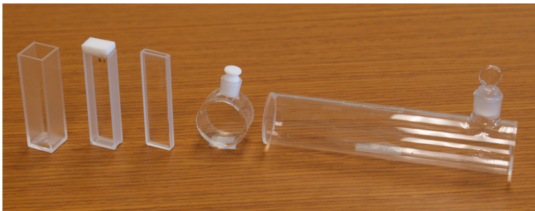
Figure 10.30 Examples of sample cells for UV/Vis spectroscopy. From left to right (with path lengths in parentheses): rectangular plastic cuvette (10.0 mm), rectangular quartz cuvette (5.000 mm), rectangular quartz cuvette (1.000 mm), cylindrical quartz cuvette (10.00 mm), cylindrical glass cuvette with quartz windows (100.0 mm). Cells often are available as a matched pair, which is important when using a double-beam instrument.
