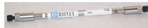
Figure 12.39 Typical packed column for HPLC. This particular column has an internal diameter of 4.6 mm and a length of 150 mm, and is packed with 5 \mu\text{m} particles coated with stationary phase.
