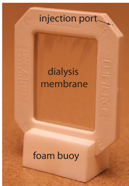
Figure 7.14 Example of a dialysis cassette. The dialysis membrane in this unit has a molecular weight cut-off of 10 000 g/mol. Two sheets of the membrane are separated by a gasket and held in place by the plastic frame. Four ports, one of which is labeled, provide a means for injecting the sample between the dialysis membranes. The cassette is inverted and submerged in a beaker that contains the external solution. A foam buoy, used as a stand in the photo, serves as a float so that the unit remains suspended in the external solution. The external solution is stirred using a stir bar, and usually replaced several times during dialysis. When dialysis is complete, the solution in the cassette is removed through an injection port.
