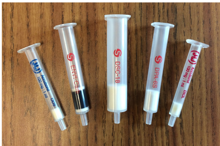
Figure 7.22 Selection of solid phase extraction cartridges for liquid samples. The solid adsorbent is the white or black material in each cartridge. From left-to-right, the adsorbent materials are octadecylsilane, carbon, octadecylsilane, polyamide resin, and diol; see Table 7.8 for additional details. The size of the cartridges dictates the volume of sample used; from left-to-right, these cartridges use samples of 1 mL, 3 mL, 6 mL, 3 mL, and 1 mL.
