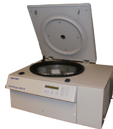
Figure 7.15 Bench-top centrifuge capable of reaching speeds up to 14 000 rpm and centrifugal forces of 20\,800 \times g . This particular centrifuge is refrigerated, allowing samples to be cooled to temperatures as low as -4^{\circ}\text{C} .
