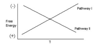
Figure 1:  $\Delta G^o$  as a function of temperature for two pathways leading to the formation of SO<sub>3</sub>(g).
